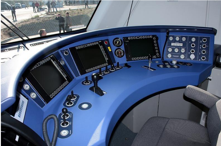
Bombardier: Talent 2 driver's cab control panel
